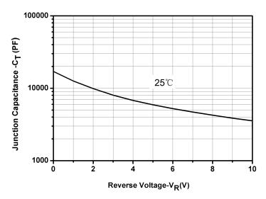
Fig.3-Capacitance vs. Reverse Voltage
